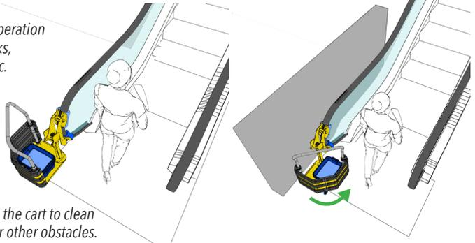
*The unique swivel mount allows the cart to clean handrails directly next to walls or other obstacles.*
